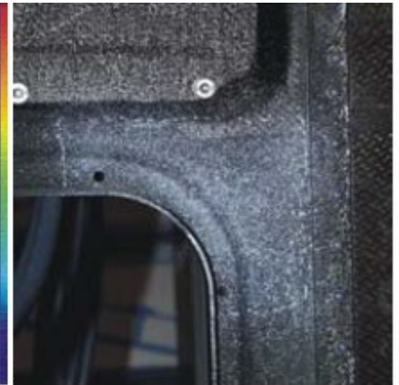
Deformation analysis on the corner of a helicopter structure (carbon fibre reinforced plastics)
